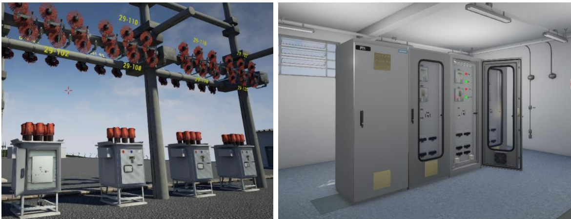
Figure 1. 3D models for low voltage circuit breaker and disconnector (left) and details of an existing panel (right)
